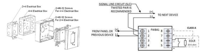
The SLC can only accommodate a max. 6 FW841, each FW841 counts for 35-unit loads.
