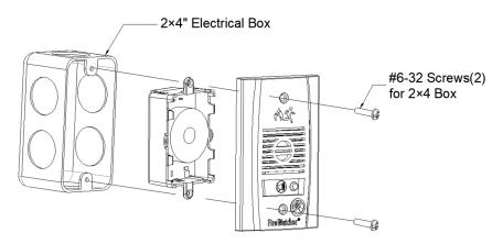
Mini horns can be used with 12 AWG to 18 AWG. Set the sound output level to the desired settings. Using the setting switch
