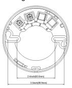
Detector base FW500 can be used with 12 AWG to 18 AWG.
